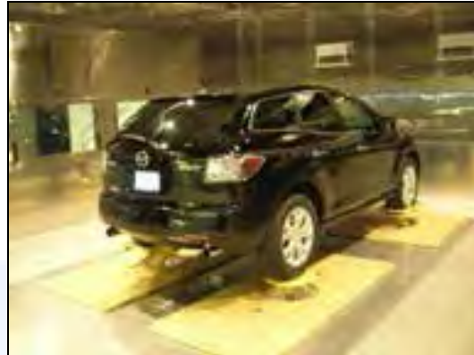
MTS Road Simulator in Weiss Environmental Chamber
