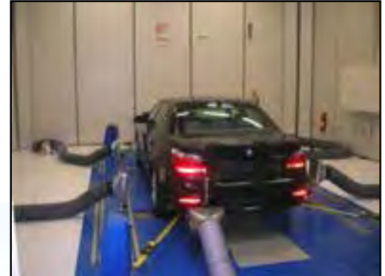
4-Wheel Chassis Dynamometer in Anechoic Chamber
